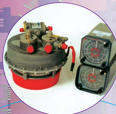
Pressurization Valves and Controllers
